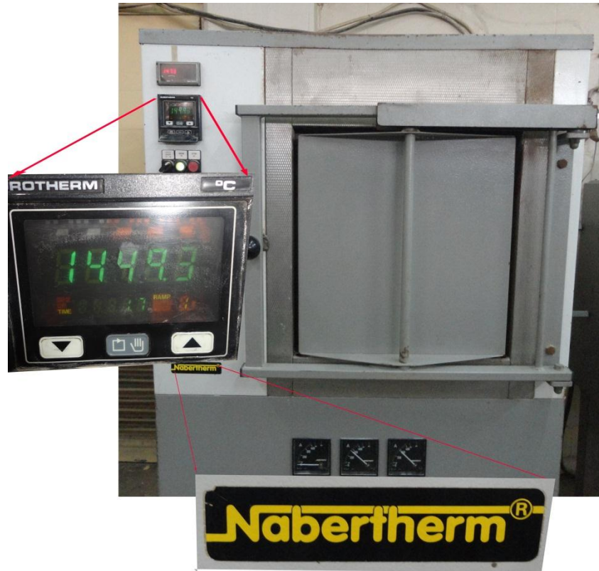
Figure 1-13: Oven that burning raw materials for manufacturing clinker in 1450°C.
